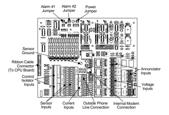
Figure 2-5: I/O Circuit Board
